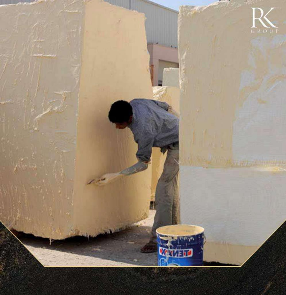
Sourcing of high quality blocks minimises the processing requirement. As a standard practice, we apply superior grade woven roving (WR-600 GSM) Fibre Net with the help of Tenax Marble Glue for block reinforcement.
